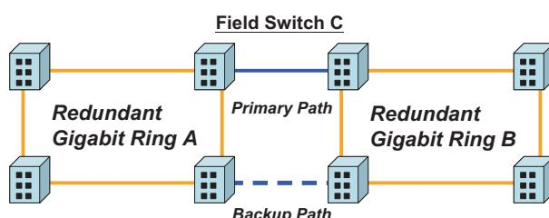
In this figure, ring coupling is illustrated with two lines connecting Ring A and Ring B. One line is the primary path, and the other is a redundant backup path. Field Switch C needs an additional gigabit port to build these two paths, for a total of three gigabit ports for ring coupling, or four gigabit ports if an additional uplink port with the core switch is needed.
